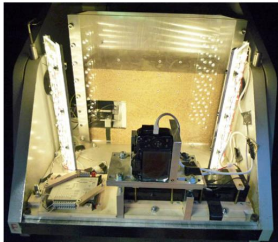
Fig. 19: Model assembly of a centrifuge experiment [Idinger et al., 2011]
