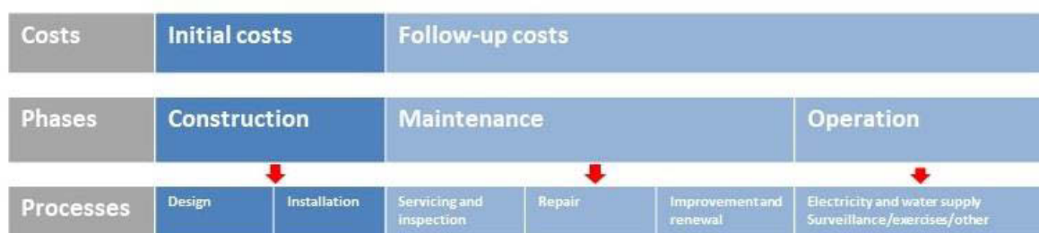
Figure 2: Lifecycle phases of tunnel equipment 6
